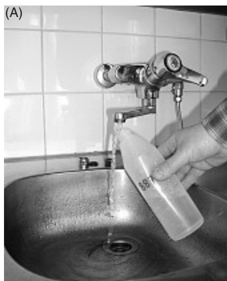
Fig. 5. Sampling from a water tap (A) and directly from a well (B).
